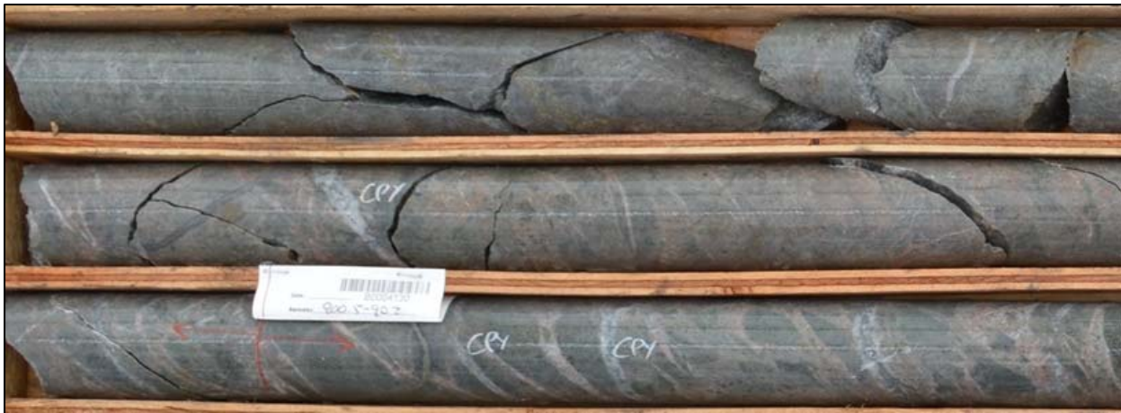
FIGURE 7.13 CORE PHOTOGRAPH OF A PINK ALKALI FELDSPAR-RICH INTRUSIVE CONTACT BRECCIA ZONE (GS-20-80, 900.0 M)
