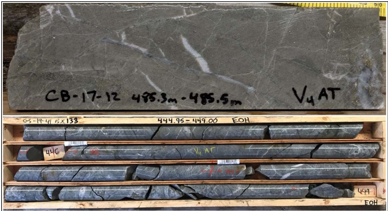
FIGURE 7.11 EXAMPLES OF A LATITE ASH TUFF 'V4AT' FROM THE GS SERIES FINE-GRAINED UNIT
