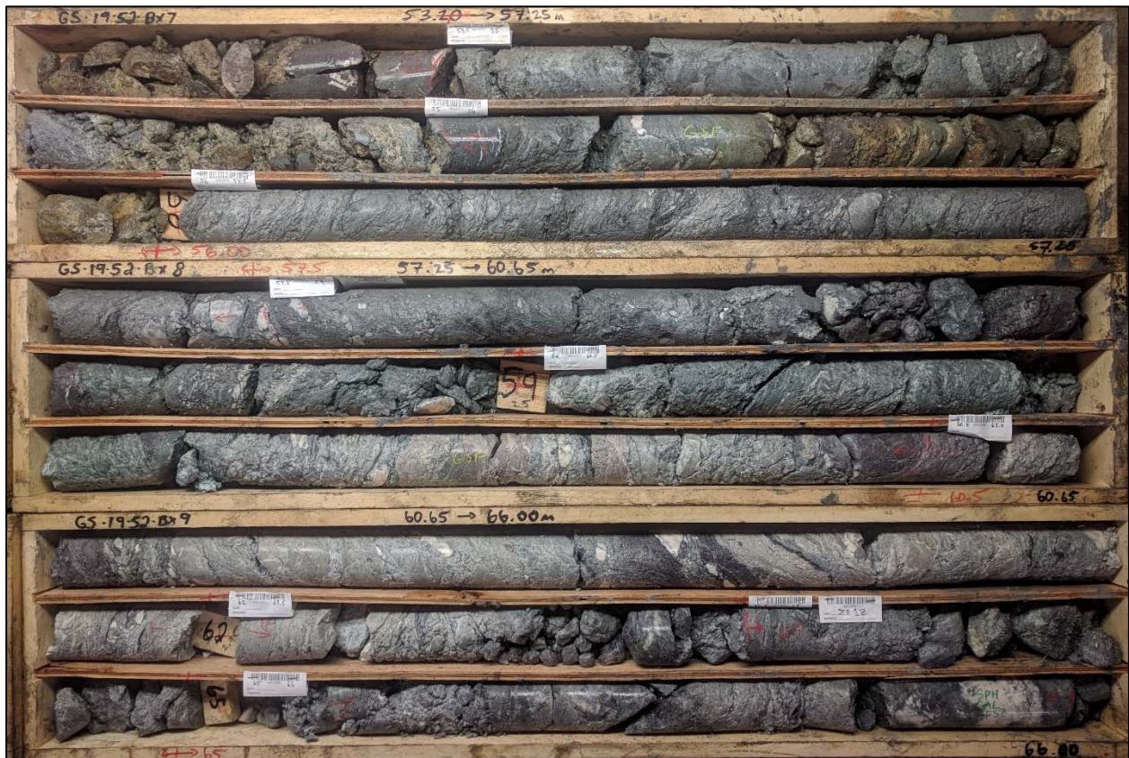
FIGURE 7.8 CORE PHOTOGRAPH FROM DRILL HOLE GS-19-52 (53.20 M TO 66.00 M) OF A TYPICAL GOUGE-RICH TTF1 INTERCEPT
