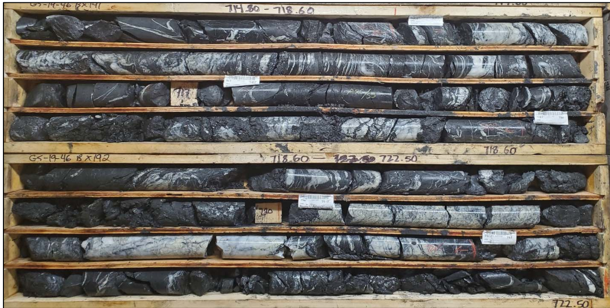
FIGURE 7.12 FOOTWALL SERIES CARBONACEOUS SILTSTONE AND MUDSTONE INTERBEDDED WITH PALE GREY-BEIGE STRONGLY CARBONATE-ALTERED TECTONIC BRECCIA FROM DRILL HOLE GS-19-46
